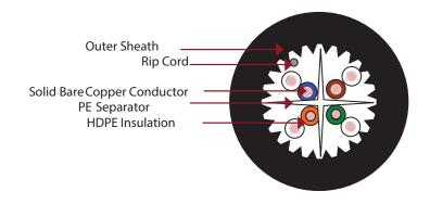
Conductor 23 AWG Solid Bare Copper
